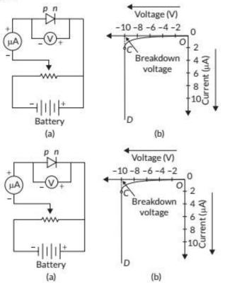
In reverse biased, the applied voltage supports the flow of minority charge carriers across the junction. So, a very small current flows across the junction due to minority charge carriers.
