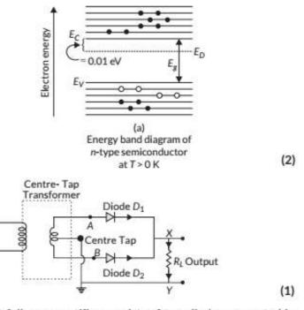
A full wave rectifier consists of two diodes connected in parallel across the ends of secondary winding of a center tapped step down transformer. The load resistance  $R_L$ is connected across secondary winding and the diodes In *n*-type extrinsic semiconductors, the number of free electrons in conductors band is much more than number of holes in valence band. The donor energy level lies just below the conduction band. Here the majority charge carriers are electrons. (2)
