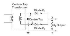
A full wave rectifier consists of two diodes connected in parallel across the ends of secondary winding of a center tapped step down transformer. The load resistance  $R_L$ is connected across secondary winding and the diodes between A and B as shown in the circuit.
