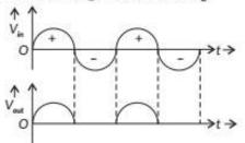
During negative half cycle of input a.c., end A of the secondary winding becomes negative and end B becomes positive. Thus, diode D becomes reverse biased and does not conduct any current. So, no current flows in the circuit. Since electric current flows through load  $R_L$  only during positive half cycle, in one direction only *i.e.*, from A to B, so d.c. is obtained across  $R_L$ .
