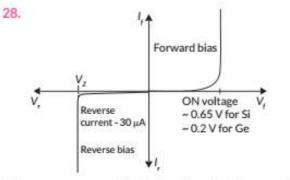
The reverse current is due to minority charge carriers and even a small voltage is sufficient to sweep the minority carriers from one side of the junction to the other side of the junction. Here the current is not limited by the magnitude of the applied voltage but is limited due to the concentration of the minority carrier on either side of the junction.
