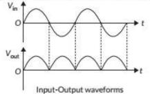
Since in both the half cycles of input a.c., electric current through load  $R_L$  flows in the same direction, so d.c. is obtained across  $R_L$ . Although direction of electric current through  $R_L$  remains same, but its magnitude changes with time, so it is called pulsating d.c.
