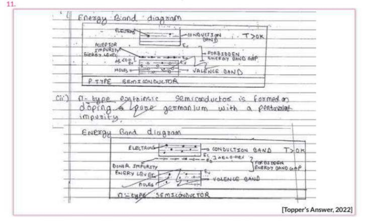
12. Intrinsic semiconductors have very small conductivity at room temperature. When certain impurities in small amount (≈ 1 part per million) are added to an intrinsic semiconductor, electrical conductivity of doped semiconductor increases to a great extent and made it useful in many practical applications. Pentavalent atoms and trivalent atoms are used for doping Ge/Si. Pentavalent atoms such as – As and Sb etc
