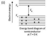
At absolute zero temperature (0 K) conduction band of semiconductor is completely empty, *i.e.*,  $\sigma = 0$ . Hence the semiconductor behaves as an insulator. At room temperature, some valence electrons acquire enough thermal energy and jump to the conduction band where they are free to conduct electricity. Thus the
