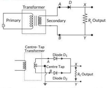
A full wave rectifier consists of two diodes connected in parallel across the ends of secondary winding of a center tapped step down transformer. The load resistance  $R_L$ is connected across secondary winding and the diodes between A and B as shown in the circuit.
