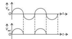
During negative half cycle of input a.c., end A of the secondary winding becomes negative and end B positive. Thus, diode D becomes reverse biased and does not conduct any current. So, no current flows in the circuit. Since electric current through load  $R_L$  flows only during positive half cycle, in one direction only *i.e.*, from A to B, so d.c. is obtained across  $R_L$ .
