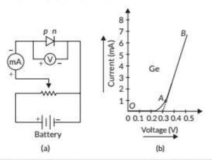
At the start when applied voltage is low, the current through the diode is almost zero. It is because of the potential barrier, which opposes the applied voltage. Till
