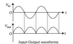
Since in both the half cycles of input a.c., electric current through load *RL* flows in the same direction, so d.c. is obtained across *RL*. Although direction of electric current through *RL* remains same, but its magnitude changes with time, so it is called pulsating d.c.
